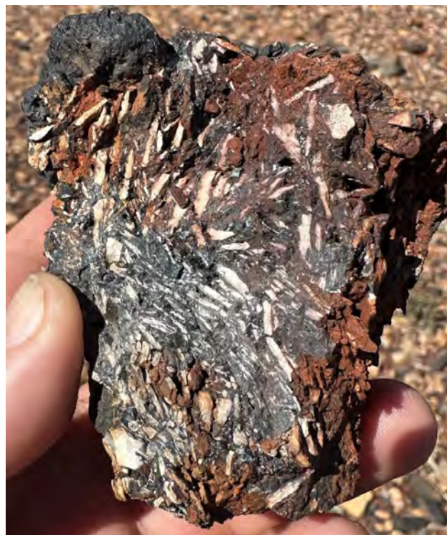
Figure 6 - Site CH87 - 390004mE 7412054mN Strongly sheared Ironstone with flattened clast
