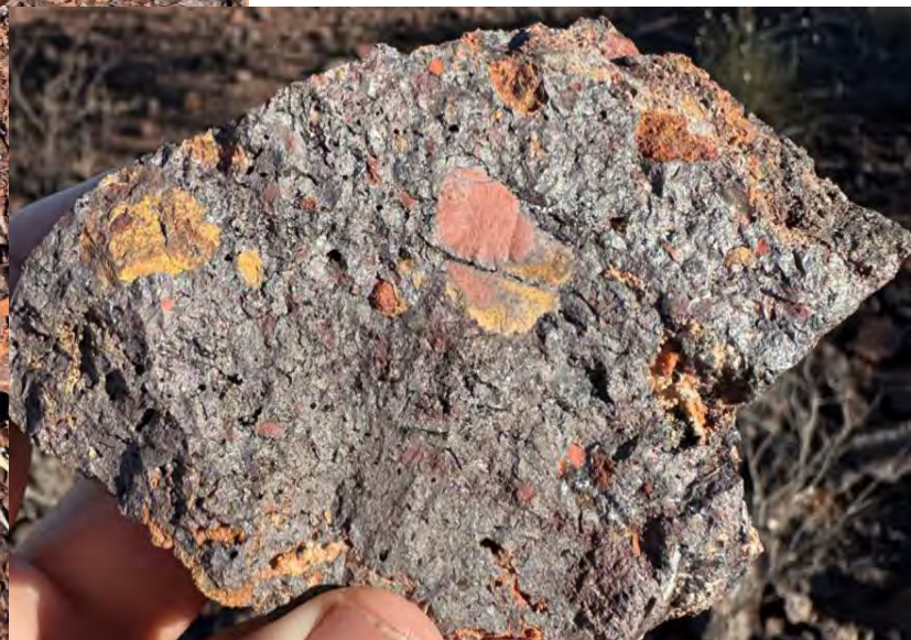
Figure 3 - Site CH101 - 390068mE 7400893mN Ironstone with metasediment clasts
