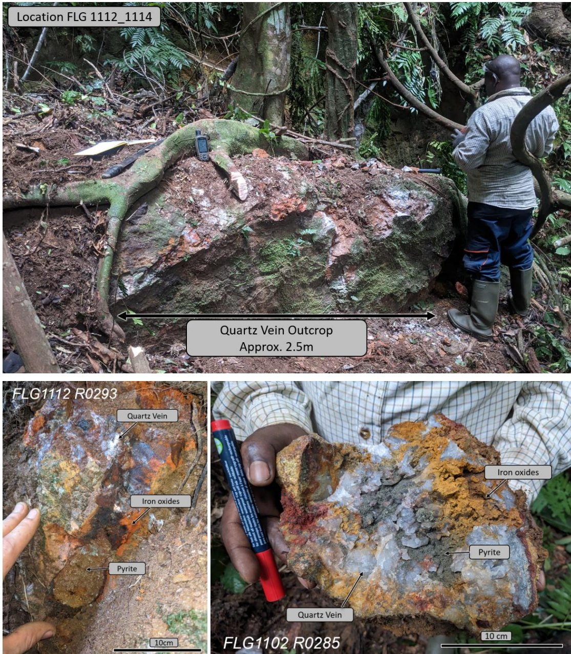
Figure 5: Examples of vein styles identified in the P6 Vein area (location FLG1112_1114). 1 (LHS: Quartz veining with up to 40% pyrite in Sample R0293; RHS: highly oxidised vuggy quartz vein with goethite (iron oxide) and pyrite ~15% Sample FLG1102 R0285)
