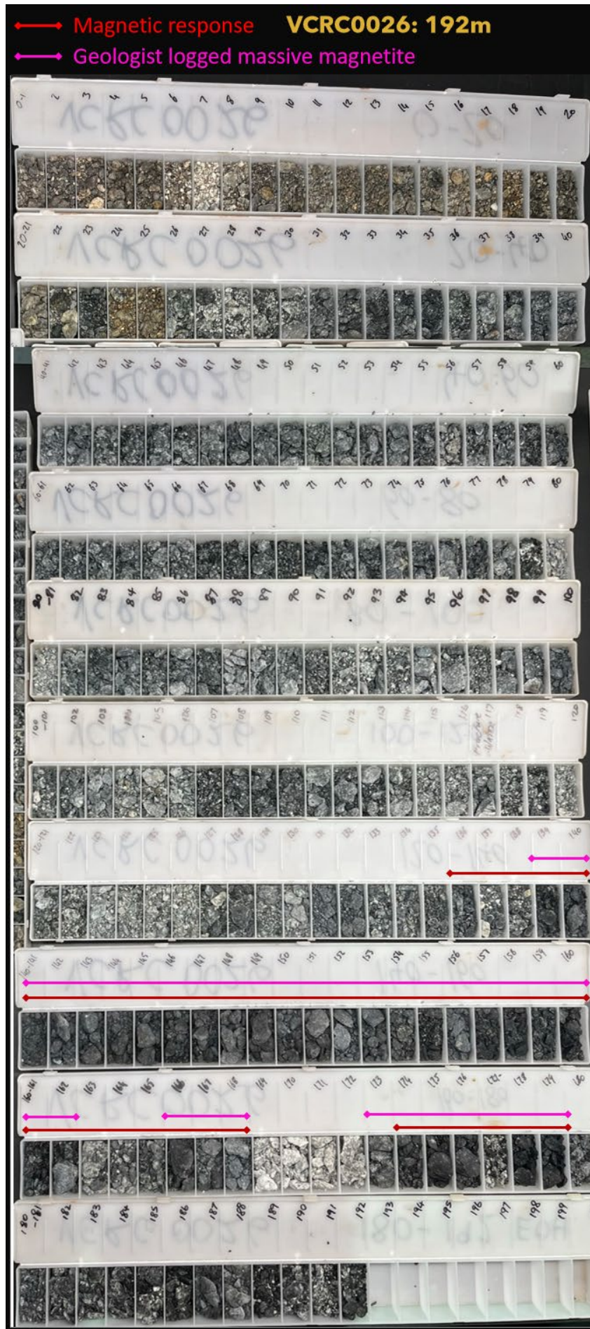
Figure 3; Drillhole chips from VCRC0026 showing the occurrence of highly magnetic material (red highlights) >6m thickness and >125 SI units \times 10^{-3} with max internal waste of consecutive 3m and zones of massive magnetite as logged by Viking geologists (pink highlights). Note the substantial thick intercept of massive magnetite from 138m to 162m downhole (see Figure 2 & Figure 4).
