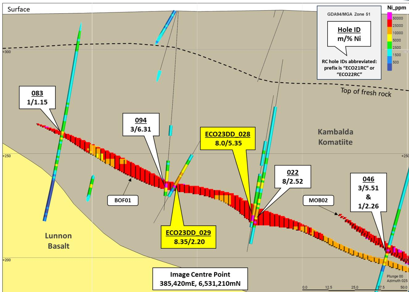
**Figure 2:** Cross section (looking NNE) through the BOF01 domain of the Baker nickel deposit illustrating the drill traces of the reported DD holes (yellow call outs) and their “twin” RC holes (Previous hole ID suffixes, where abbreviated, are “ECO21RC\_” or “ECO22RC\_”).
