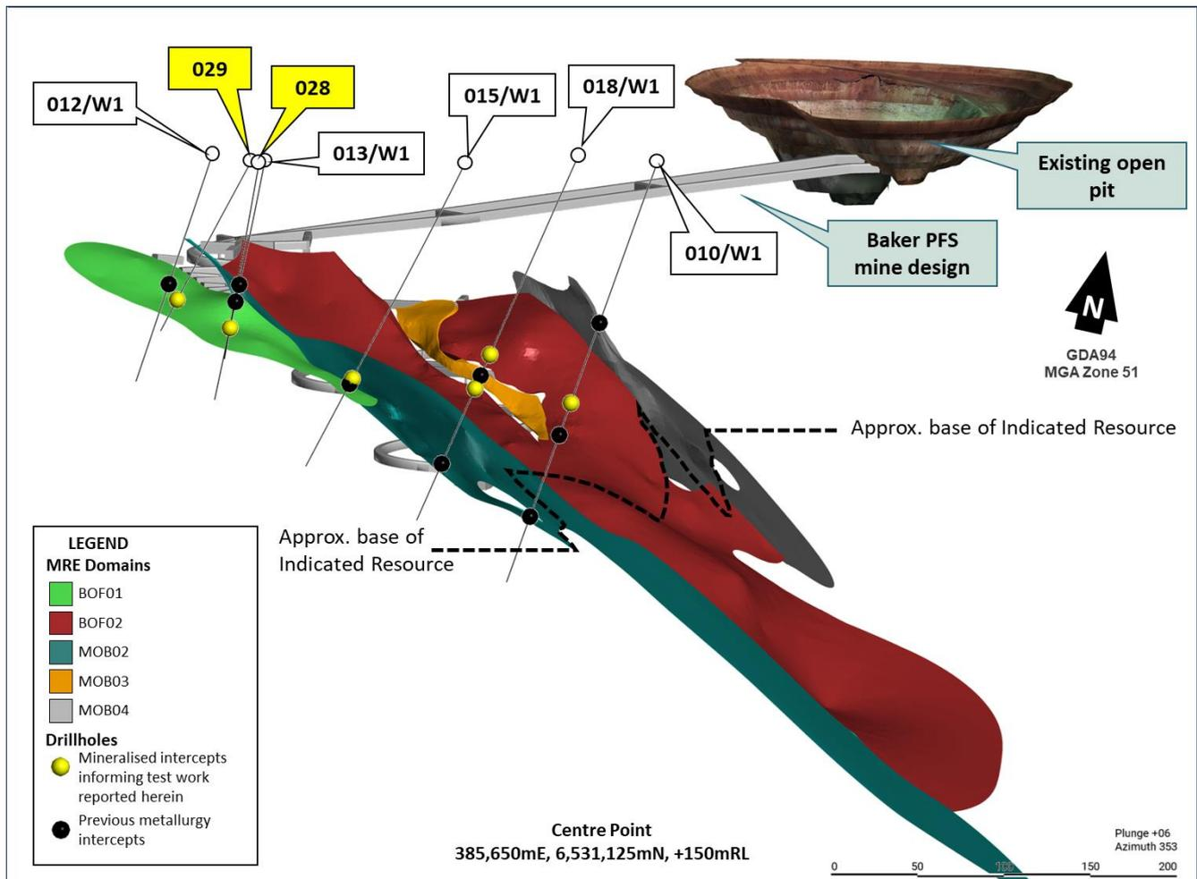
**Figure 1:** Isometric view of the Baker nickel deposit looking north illustrating pierce point of reported (yellow call outs) and previous parent and "twin" hole drill traces, December 2022 MRE geology domains<sup>4</sup> and PFS underground decline design. (Past DD hole ID suffixes, where abbreviated, are "ECO22DD\_", present DD hole ID suffixes, where abbreviated, are "ECO23DD\_")
