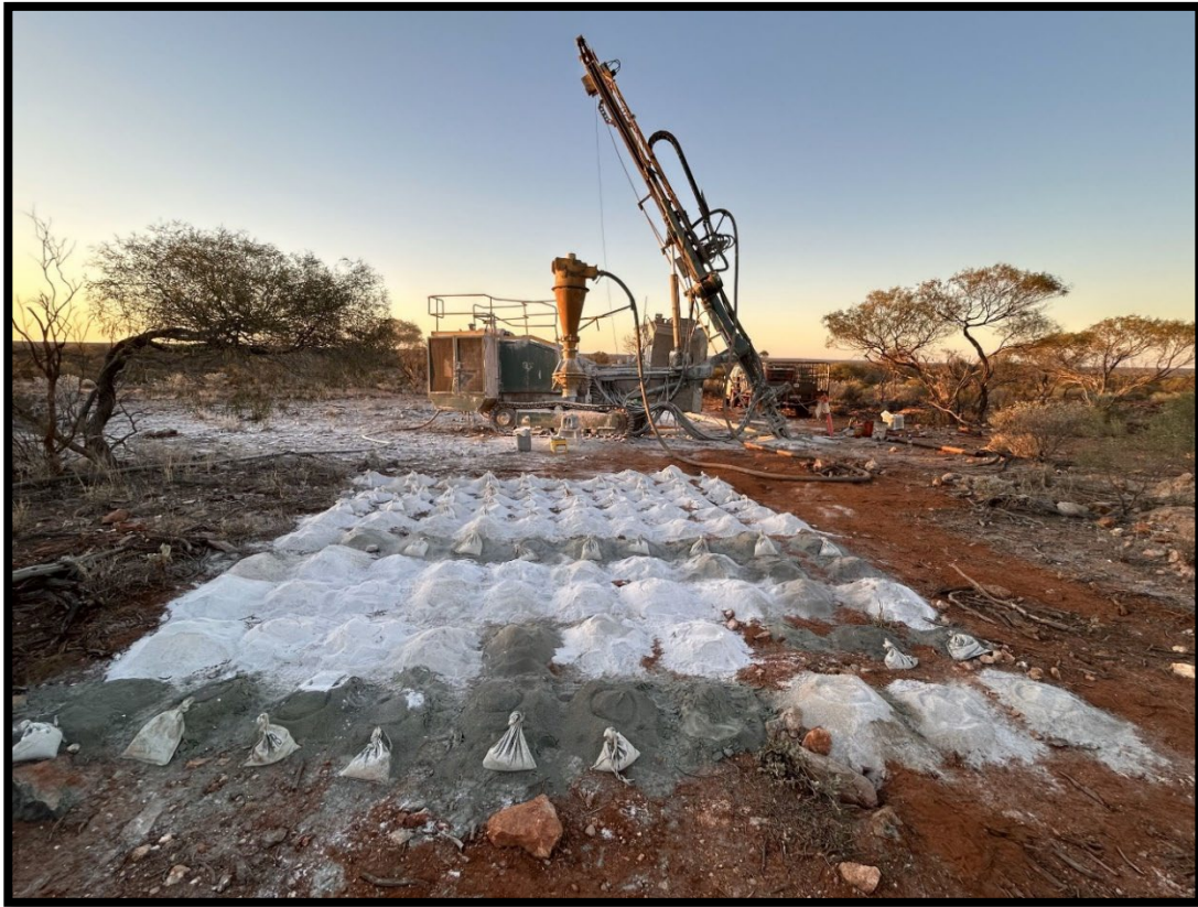
Figure 2: RC drilling at Mt Edon (hole MD23- 07) indicate thick zones (white samples), view to west
