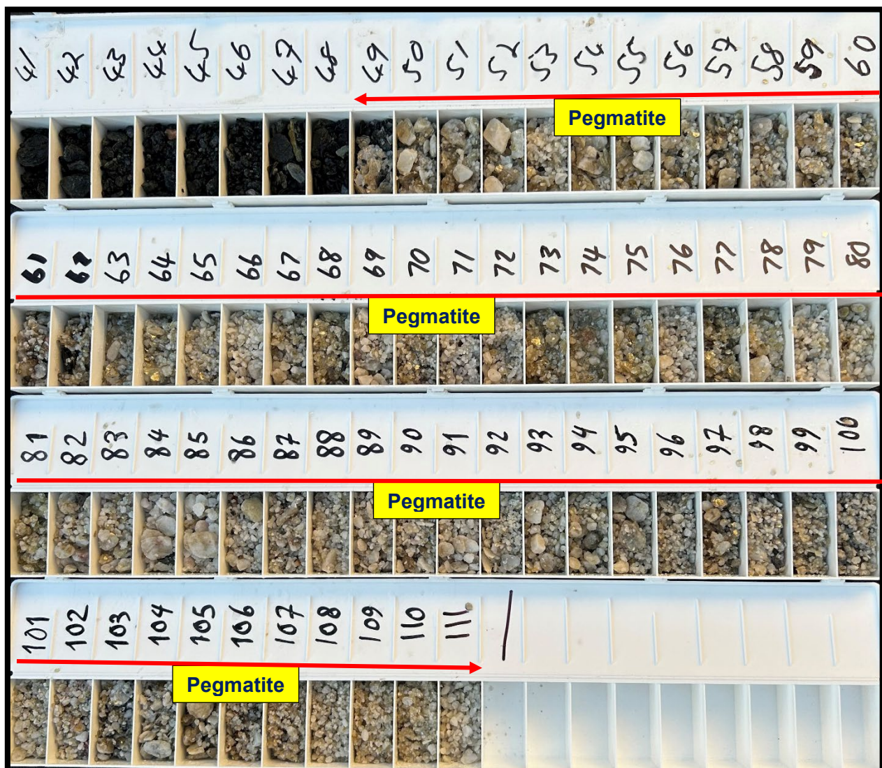
Figure 3: Chip tray for hole MD23- 07, showing thick interval 49m to 111m, remained open at depth. Well-developed mica rich zones can be seen in different intervals
