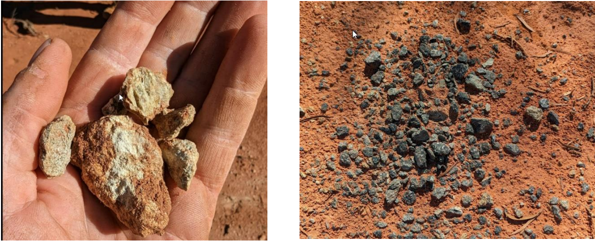
Figure 6 – Drill cuttings located by WYX geologists at BHP AC hole HWAC12 with 45m @ 0.55% Ni
