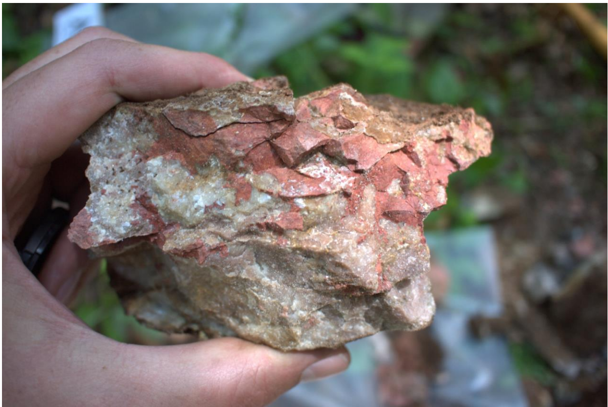
Figure 1. REE mineralisation (red mineral) in sample K042532 with assays of 35,896 ppm (3.6%) TREO and 4,706 ppm (0.5%) ppm Nb 2 O 5 from the Blue Jay prospect
