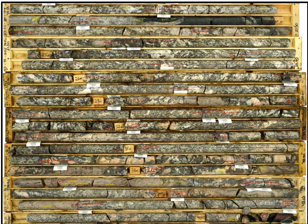
Figure 1 – 23FL-001 Core Box 27.6m @ 1.37% Li 2 O
