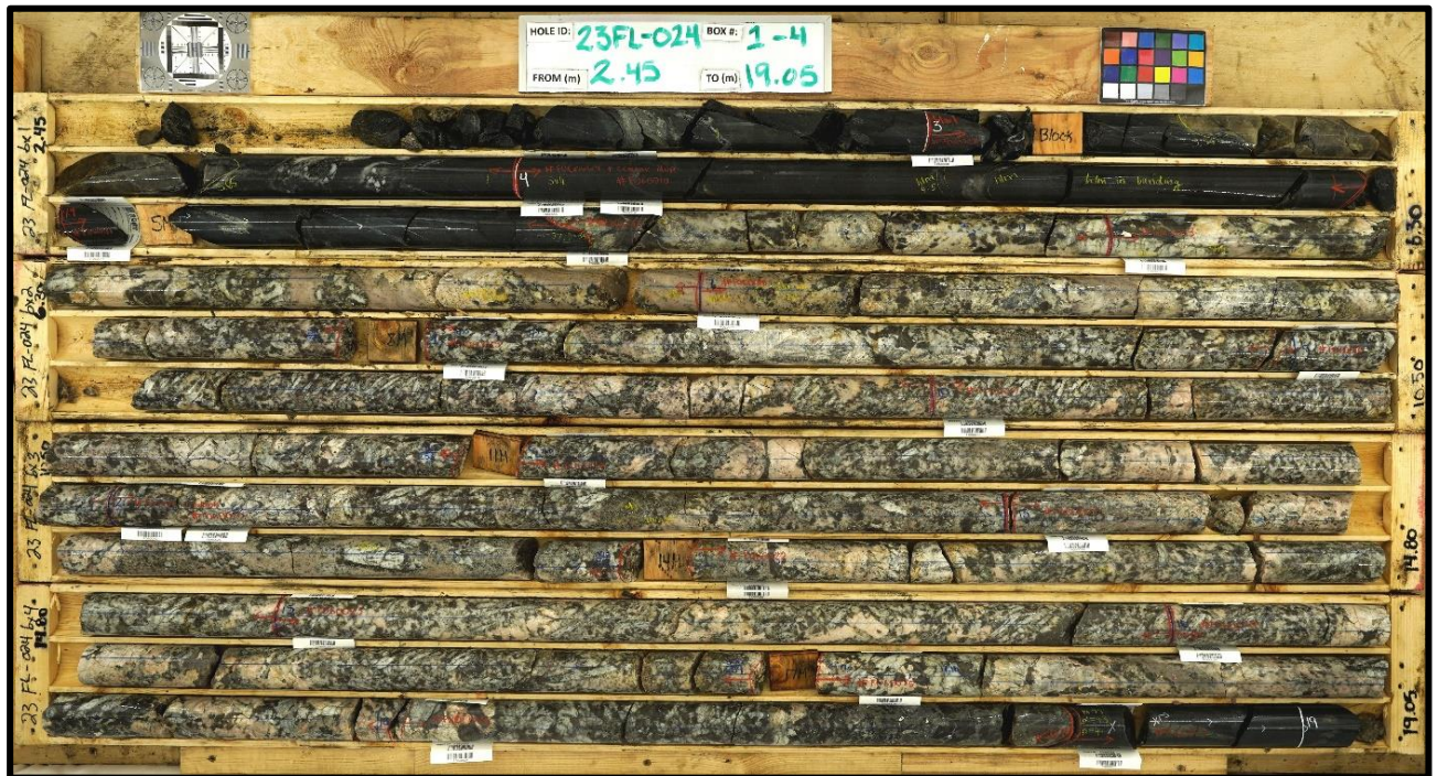
Figure 5 - 23FL-024 Core Box showing mineralised pegmatites visually estimated up to 25%
