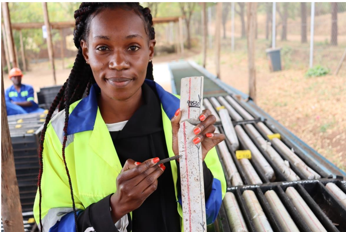
Image 2: Serah Misuku, Site Program Geologist, with a section of drill core showing textural features of monazite, strontianite and baryte (replacing original burbankite crystal pseudomorphs) at 995.3m downhole. Estimation of abundance of monazite range 0.5% to 3%.
