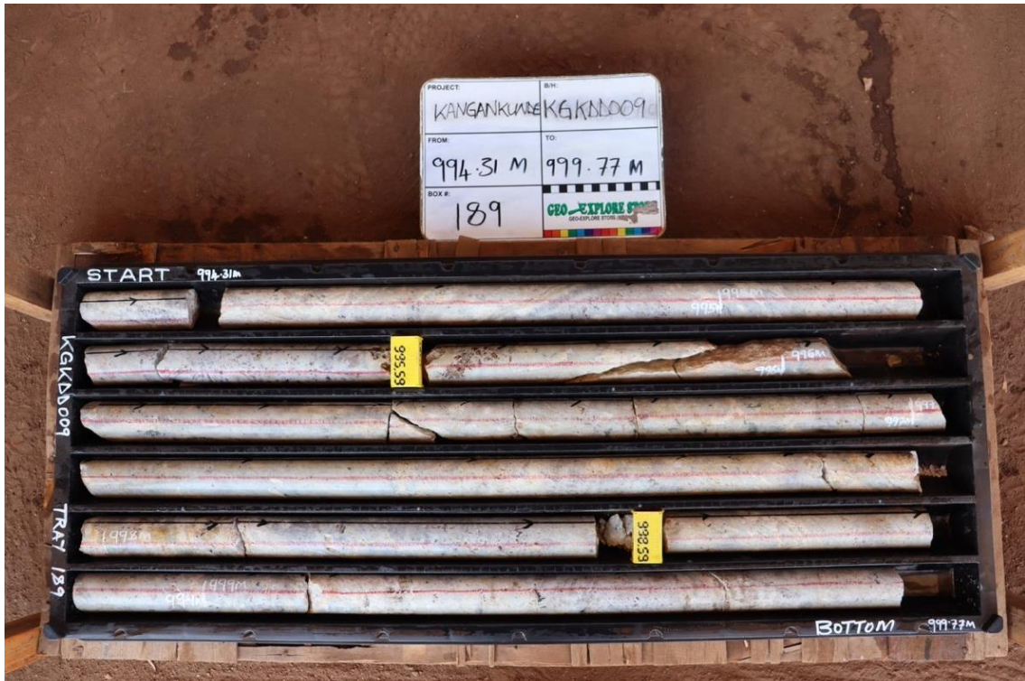
Image 1: Pieces of the drill core from KGKRC009 that appear to show the crystal texture of the monazite at depth, similar to the textural consistency of mineralisation observed at surface. Estimation of abundance of monazite range 0.5% to 3.
