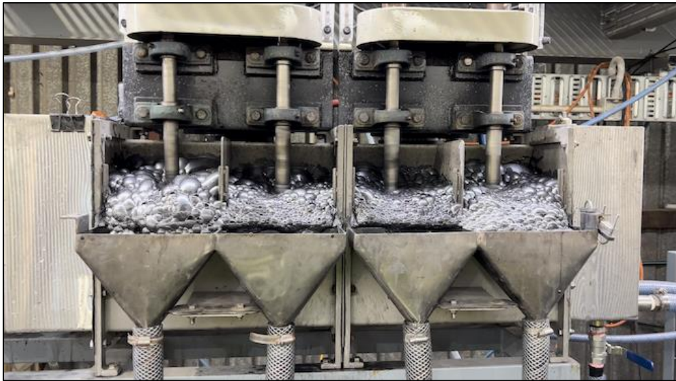
Photo 1: Flotation test work underway to produce a fine flake bulk concentrate from Kambale diamond drill core.
