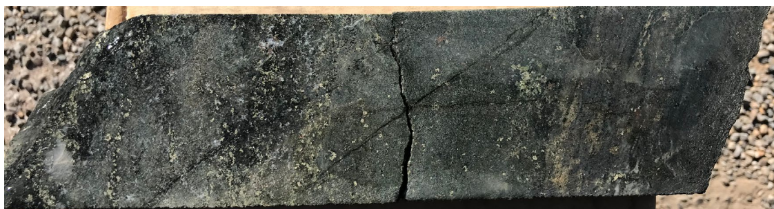
Figure 3: MMA016 drill core (235.2-235.4 m). Base metal zone below RSZ. Pervasive green alteration with shear banding, disseminated and fine stringer sulphides (1 m assay from this interval returned 2.24% Zn).
