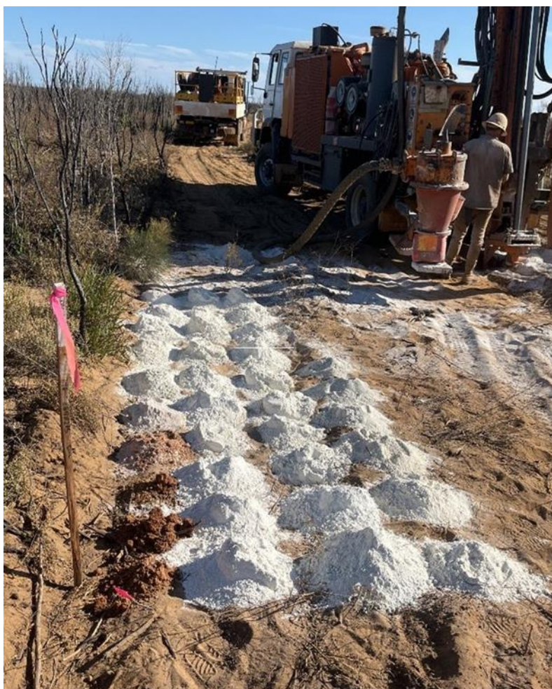
Figure 10: High quality Kaolin intersected 30m of bright white kaolin from 4m depth (KAC014).
