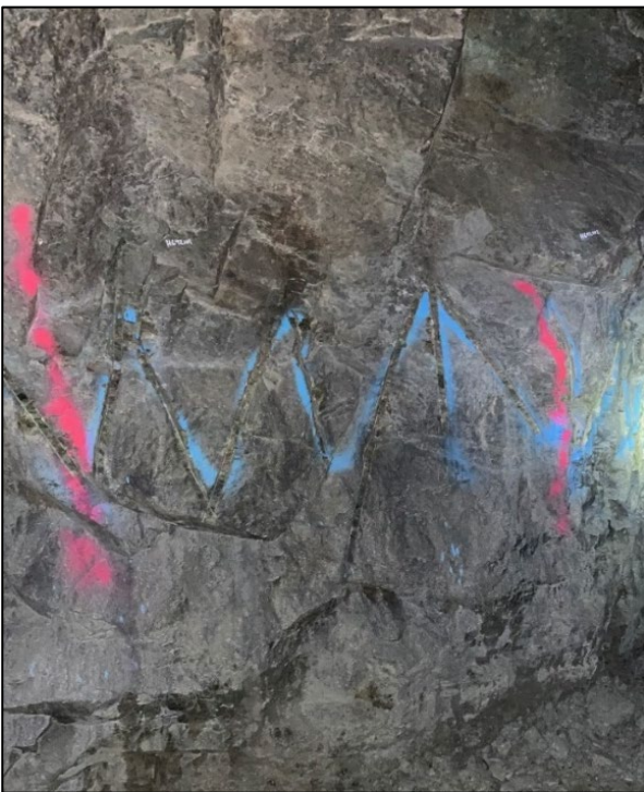
Photo 1 (Left) - Example of channel sampling of underground walls showing the "herringbone" sampling pattern. Photo 2 (Right) - Chalcopyrite rich mineralisation in channel sample in 6500-NW-002 from 9.1m to 10.7m, within a zone 32.6m long grading 2.23% Cu, 26.13g/t Ag and 0.28g/t Au
