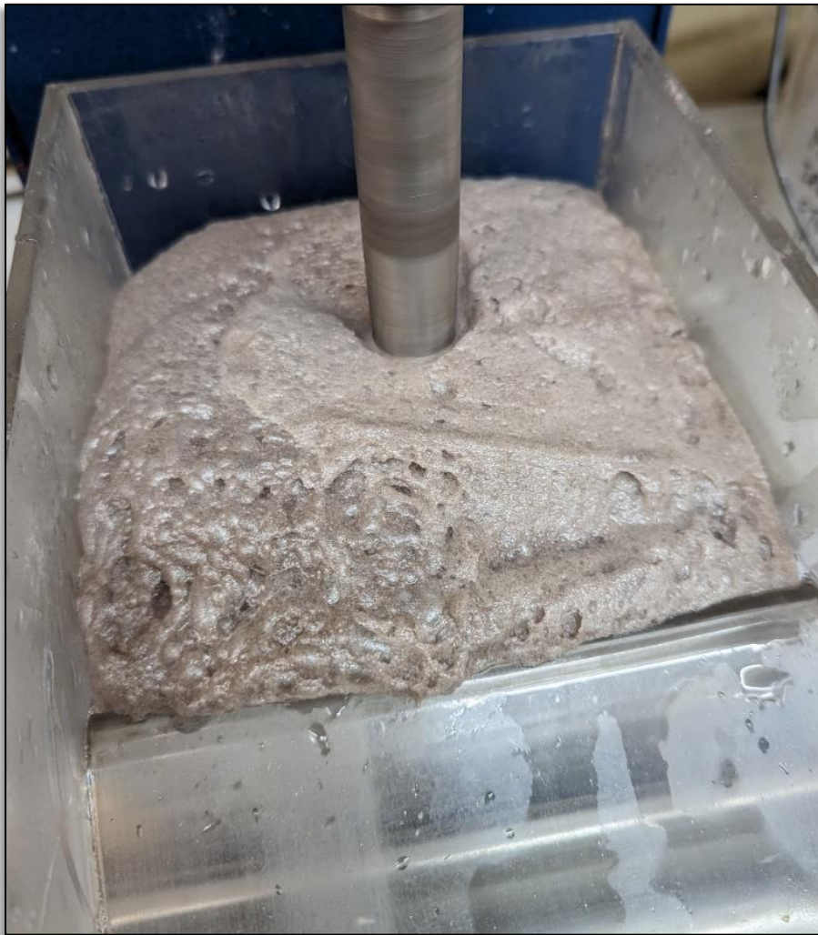
Figure 6: Mt Deans sample undergoing flotation test.
