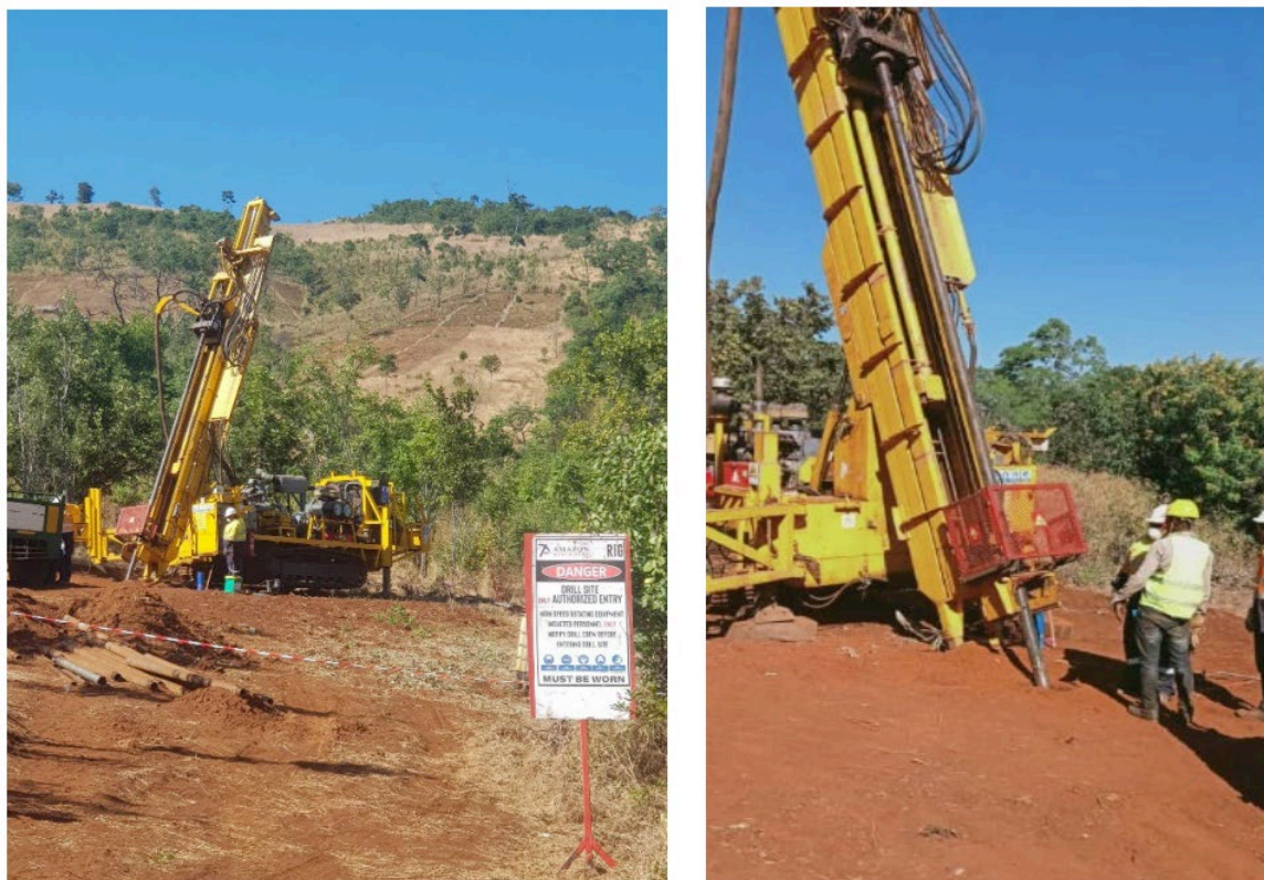
Figure 4: Reverse Circulation Drilling at the Liparamba Nickel Project
