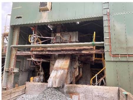
Figure 1. Old SAG discharge hopper
