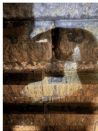
Figure 4. New and Old mill liners
