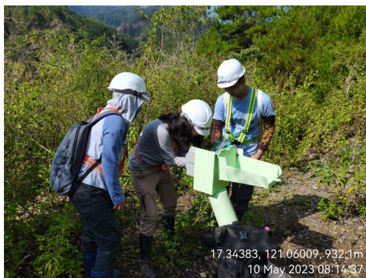
Data retrieval from vibrating wire piezometers (left) and water level reading of completed drill holes (right)
