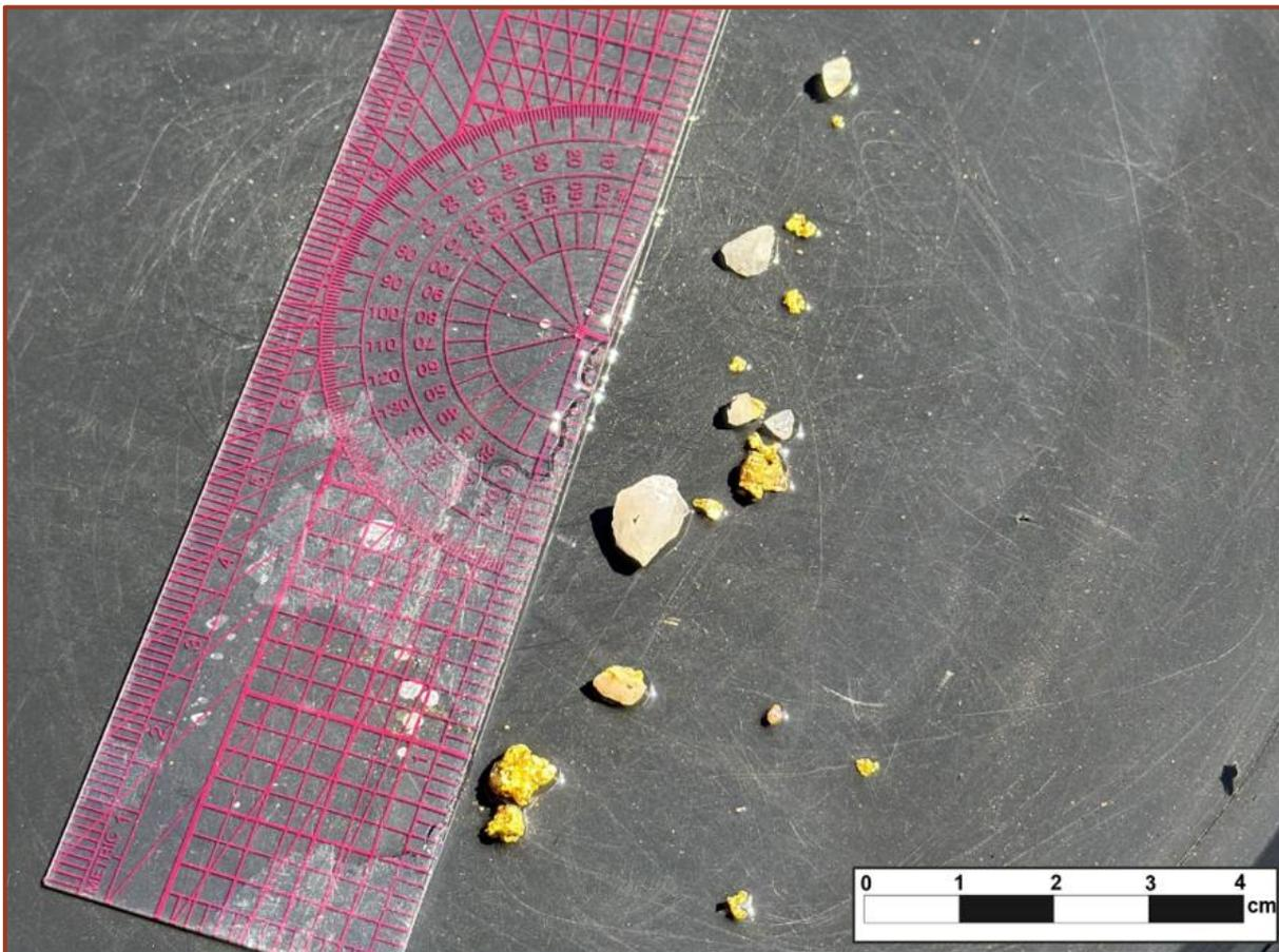
*Figure 3 – Coarse Gold Panned from EDJAC164 (27 – 28m)*
