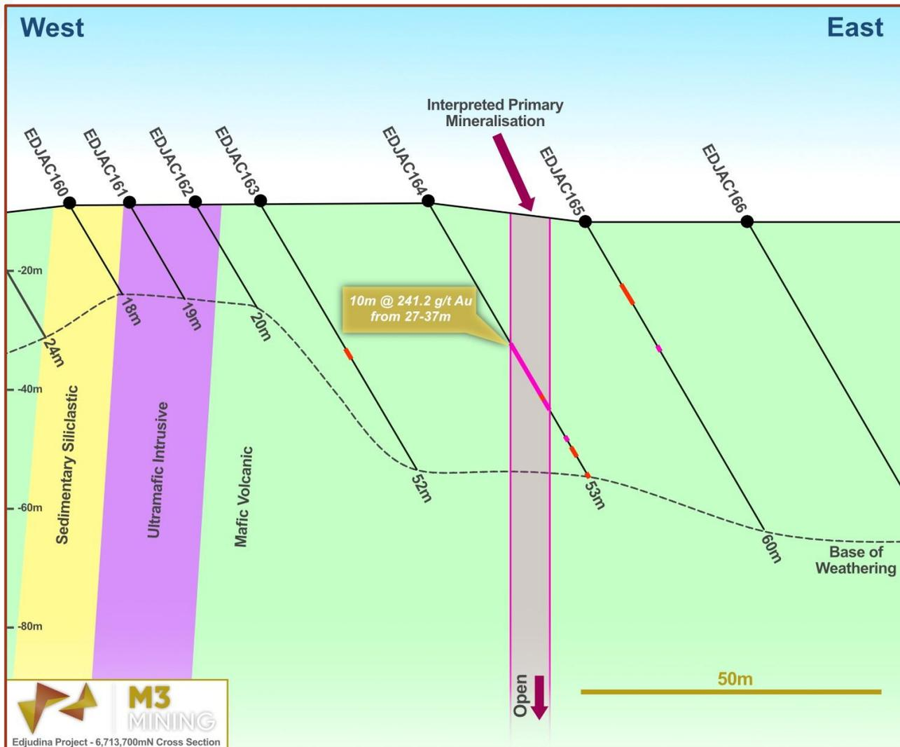
Figure 5– Cross Section of Mineralisation encountered in Drillhole EDJAC164
