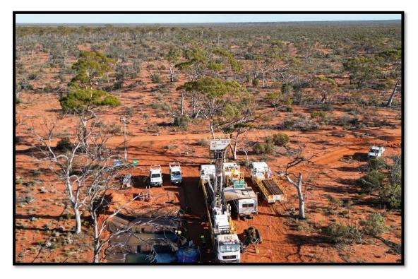
Photo 1: Diamond drillhole OCDD005 underway at Target Area B.
