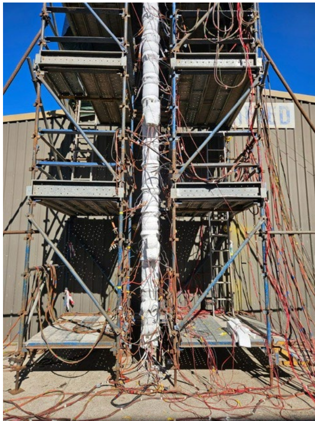
Figure 1: Heat exchanger successfully completes heat treatment prior to final assembly and delivery to site
