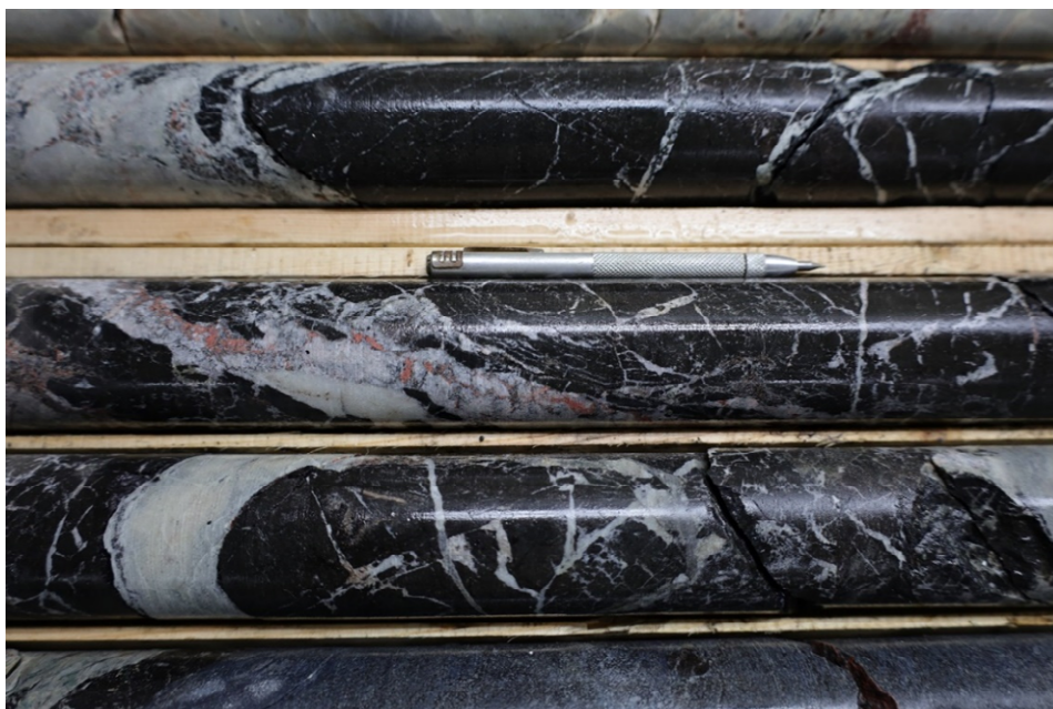
Figure 7: Diamond drill core (NQ, approximately 4.8 cm diameter) containing REE mineralisation (red coloured disseminations) within silicocarnatite host rock. Hole POM-23-01, Box 3, 39.0 – 43.5 metres downhole depth.
