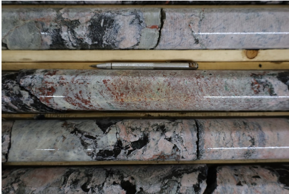
Figure 6: Diamond drill core (NQ, approximately 4.8 cm diameter) containing REE mineralisation (red coloured disseminations) within ferrocarnatite/calciocarnatite host rock. Hole POM-23-01, Box 15, 91.1 – 95.5 metres downhole depth.
