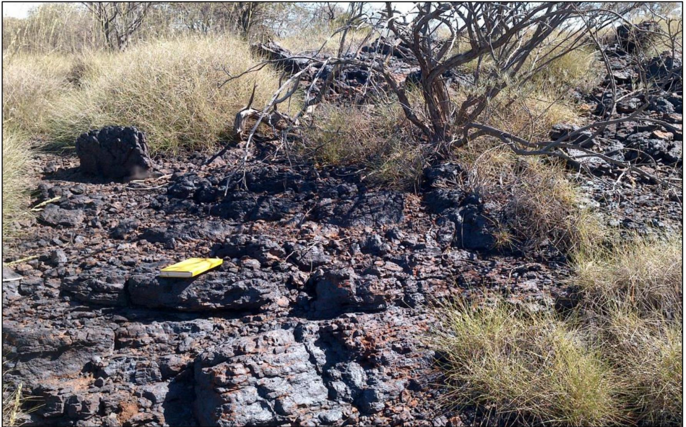
Figure 6: An example of the blocky manganese enriched shale mineralisation at KR 1 located within E46/1383.
