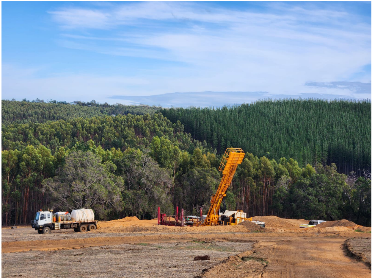
Figure 13: Diamond Drilling at Greenbushes South Project
