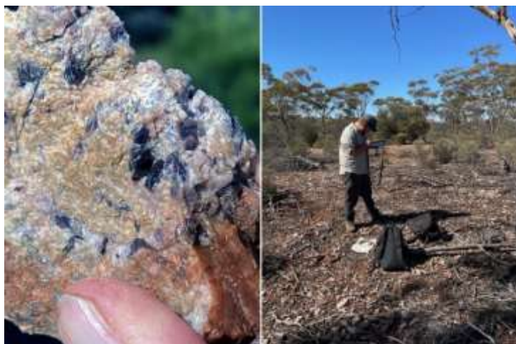
Figure 3: Rock-Chip ALY80612 with lepidolite in pegmatite (LHS), pegmatite at its field location (RHS)
