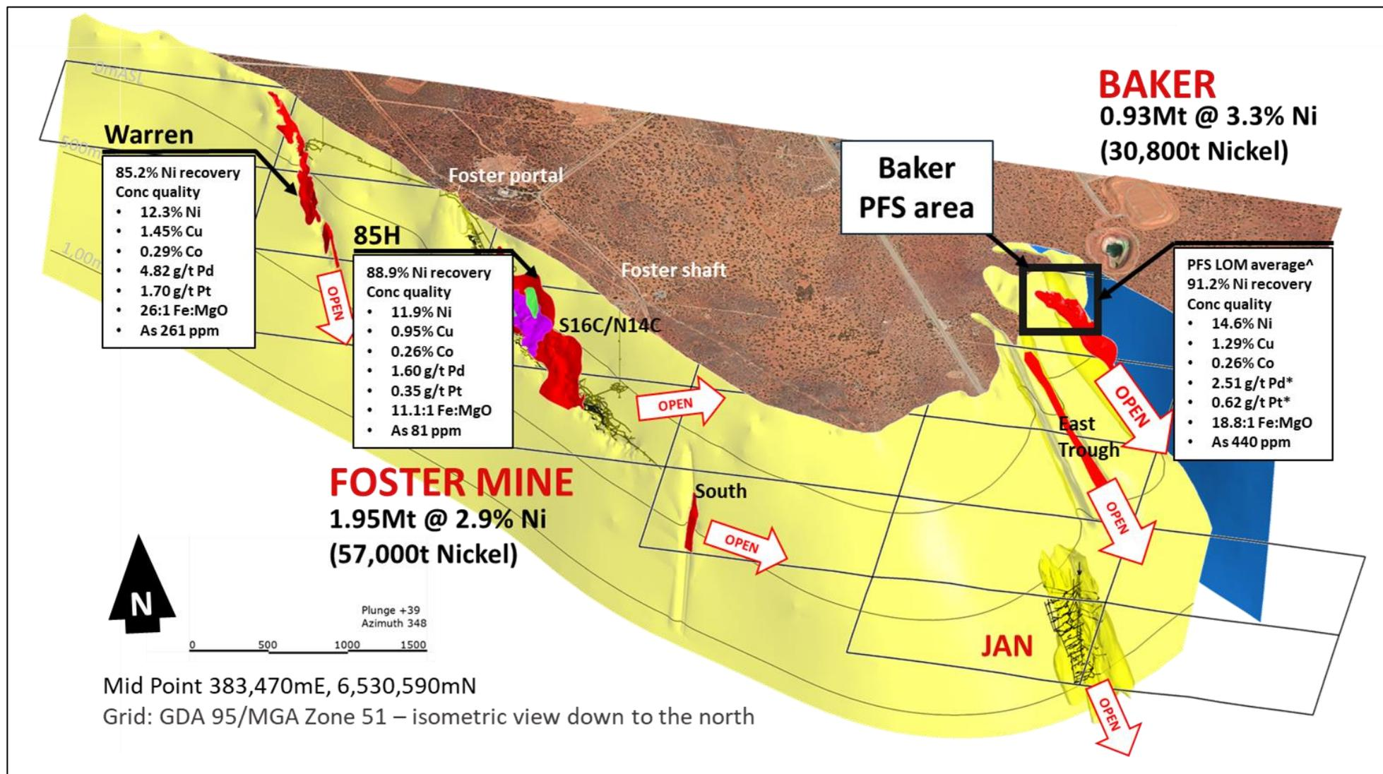
**Figure 2:** Isometric view of the Foster-Baker project at KNP, looking north illustrating MRE totals and updated<sup>8</sup> and new metallurgical testwork results.
