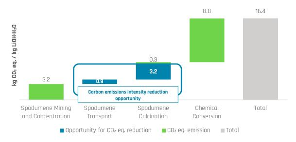
**Figure 1 -** Potential reduction in carbon emissions intensity using renewable electric calcination on site compared to shipping spodumene concentrate and processing in a conventional coal-fired calciner for lithium hydroxide production in China. <sup>4</sup>
