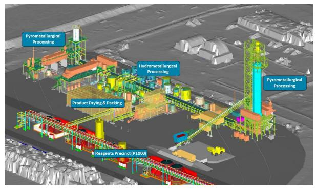
Figure 2 – Mid-Stream Demonstration Plant location and layout
