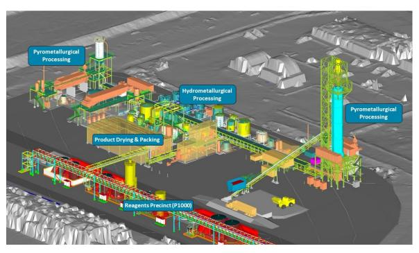
Proposed Mid-Stream Demonstration Plant schematic
