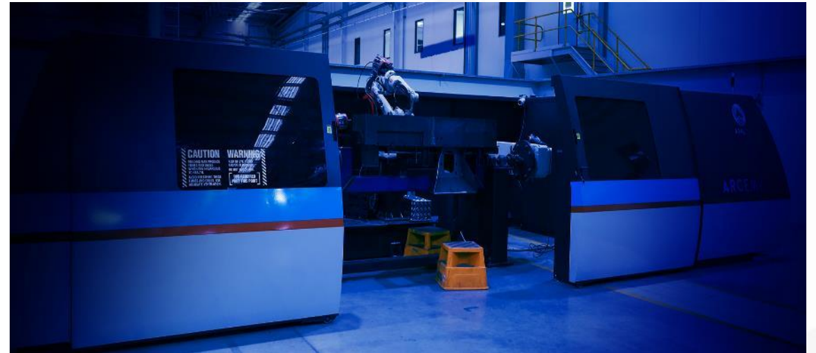
ARCEMY® is a metal 3D printer for medium to large-scale parts
