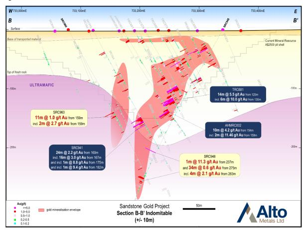
Figure 2: Indomitable section B - B'
