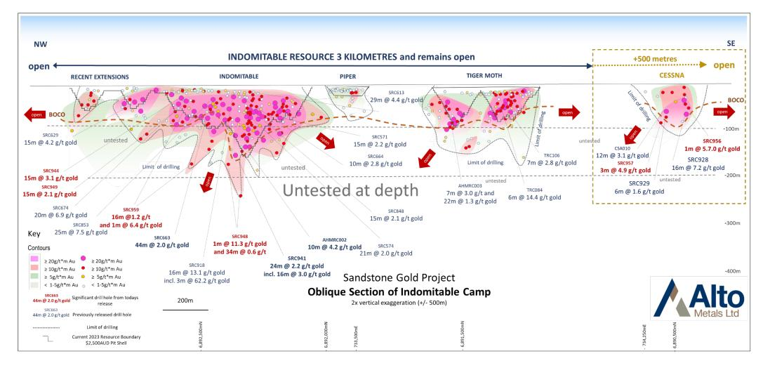
Figure 4: Oblique section of Indomitable Camp showing g/t\*m drill results
