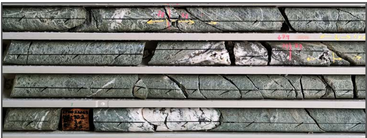
Figure 1: Gold and sulphide bearing quartz-barite veins in a zone which returned 8.5m @ 5.47g/t Au (LTDD22068).
