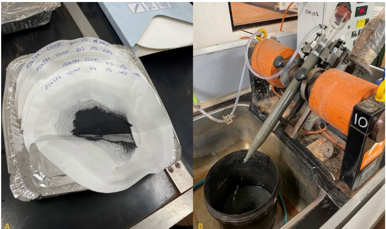
Figure 2; A) Magnetic concentrate produced using Davis Tube Wash method. B) Viking samples undergoing Davis Tube Wash testwork at ALS Metallurgy laboratories in Perth. Photos taken by Vikings Competent Person for Metallurgy, Damian Connelly from METS during visit to ALS Metallurgy laboratory to supervise testwork activities.
