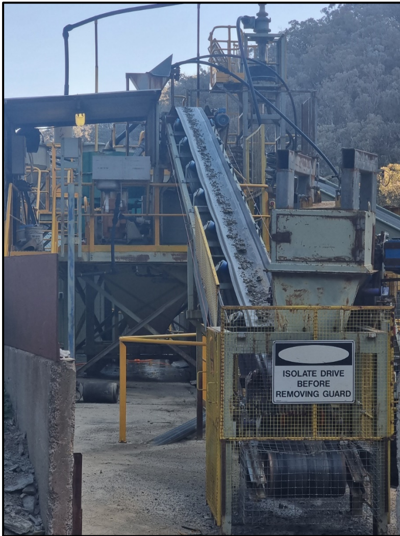
Image 1: Crushed Stockpile material being fed into the Hill End Gold Plant.
