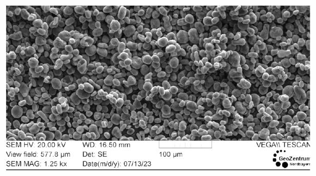
Figure 1: SEM image of Buxton's SPG15 spheronised product
