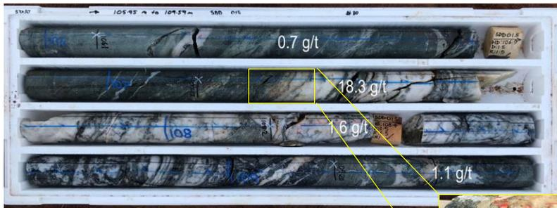
Figure A. Diamond core from SDD015 from 105.95m to 109.59m with visible gold at 107.4m in HQ (63mm diameter). SDD015 intersected a quartz-rich laminated shear vein from 107.3m to 109.2m, within a broad 28m wide zone of extensional quartz veins, with distinct haloes of coarse-grained pyrite, from 88.5m to 116.5m, Overall intercept assayed 30m @ 3.0 g/t gold, incl. 1m @ 18.3 g/t gold from 107m
