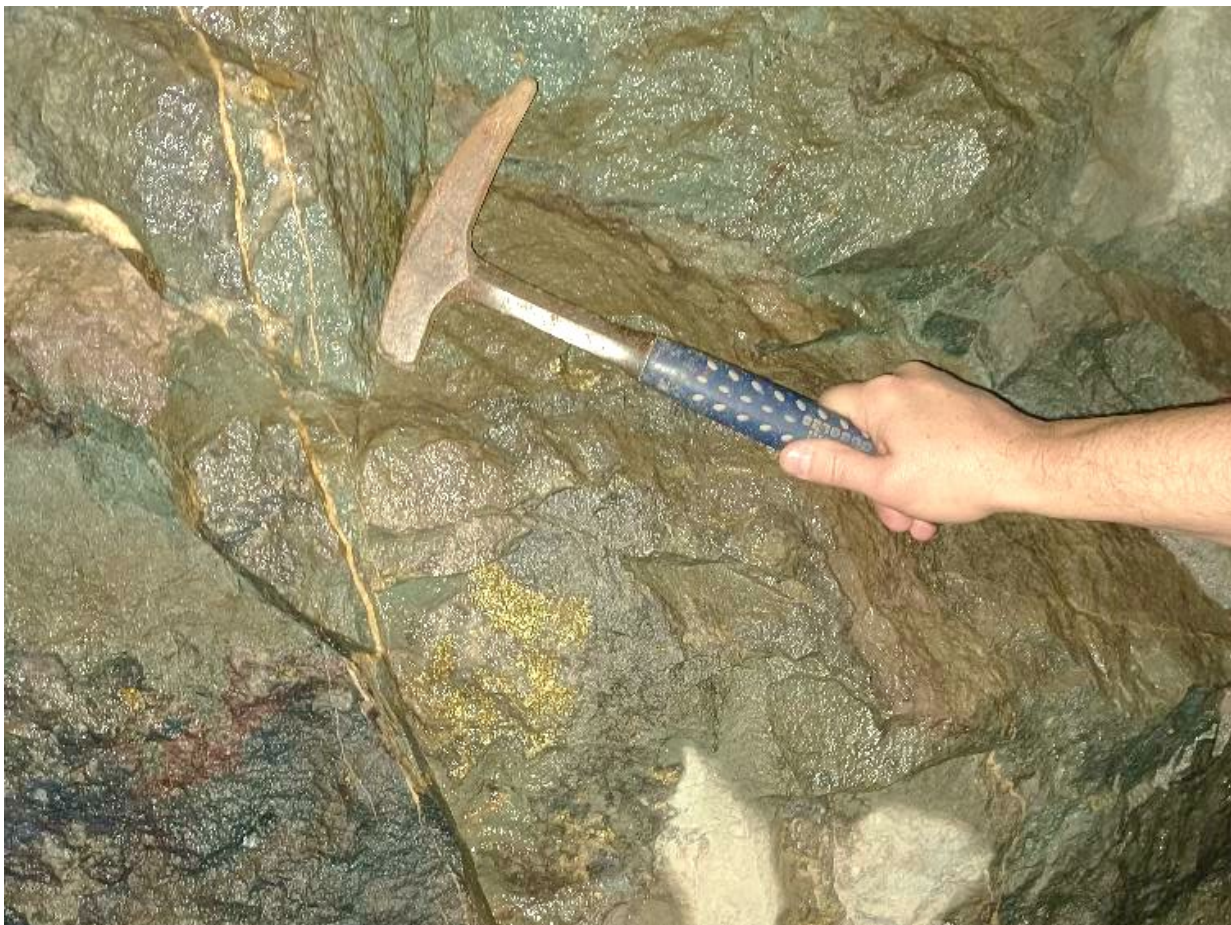
Figure 4: Chalcopryite - copper sulphide mineralisation present in historic underground workings at El Quillay
