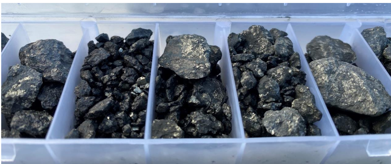
Figure 3: Sulphides in RC chips, hole ARRC001, 121 – 126m.
