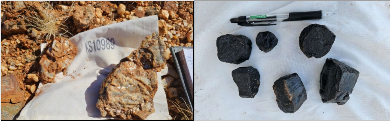
Figure 3: Photographs of typical quartz, feldspar and mica Pegmatite and the tourmaline crystals (float) found around the Lucys pegmatite area
