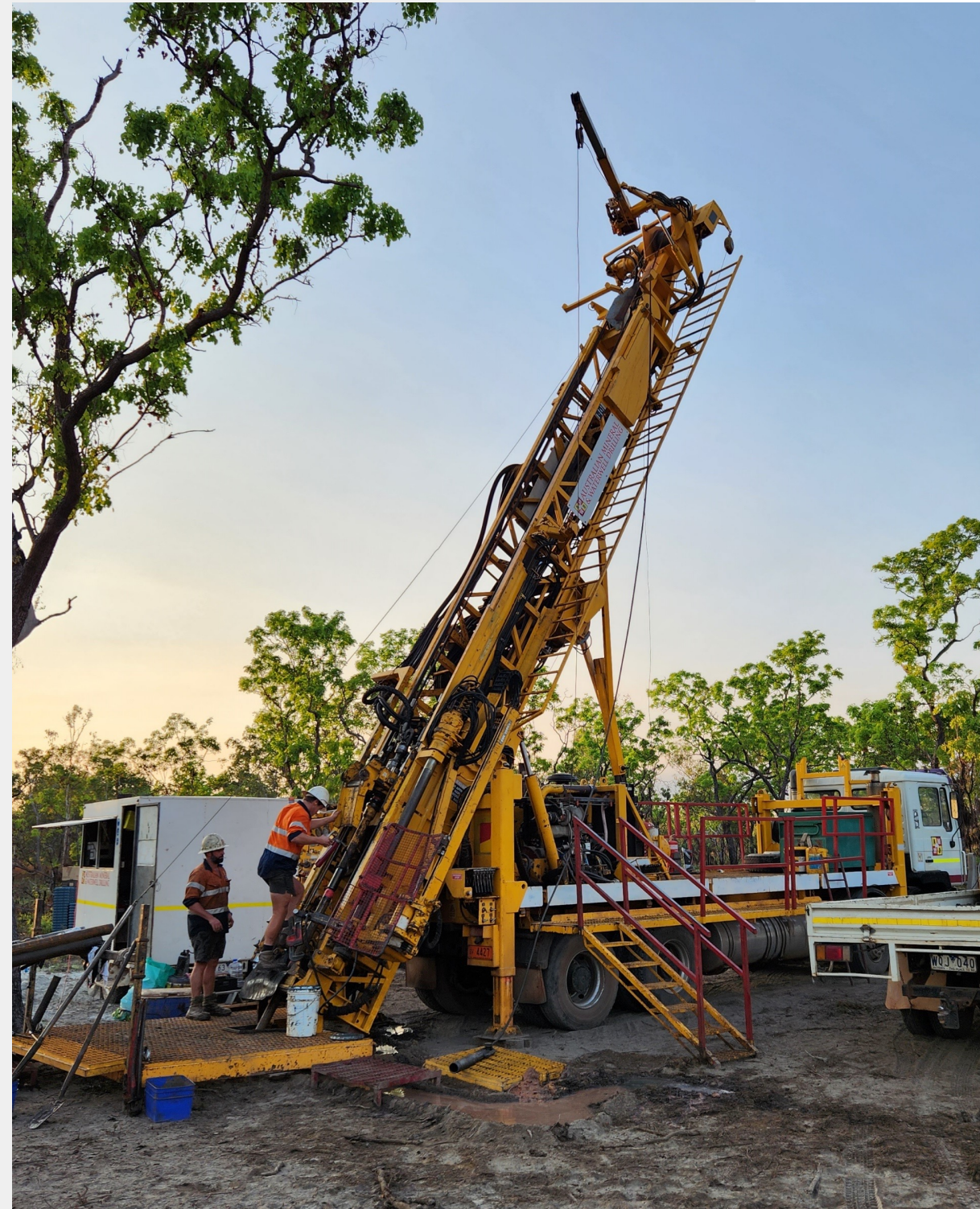
Diamond drilling at Bynoe
