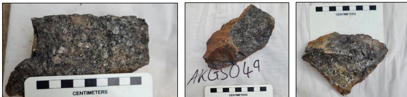
Figure 6. Rock chip samples of ultramafic intrusive rocks at the Arkun project, WA. These rocks and prospects can potentially host nickel copper PGM deposits, and follow-up fieldwork is a priority.
