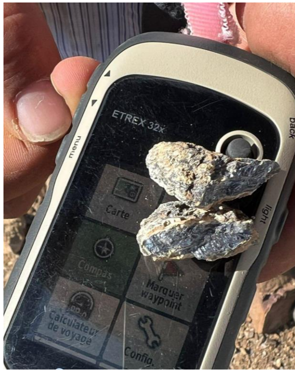
Figure 5 – Primary stibnite mineralisation from outcrop
