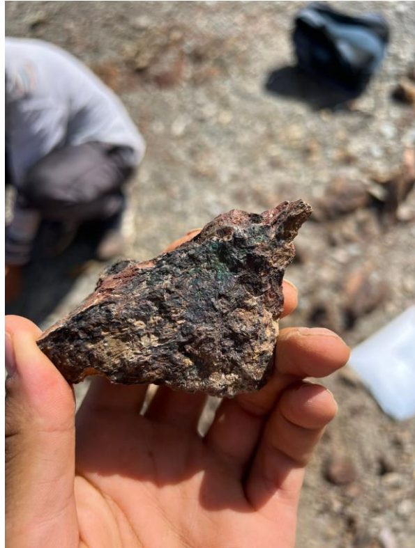
Figure 3 – Secondary copper oxides (malachite and azurite) after copper sulphide mineralisation
