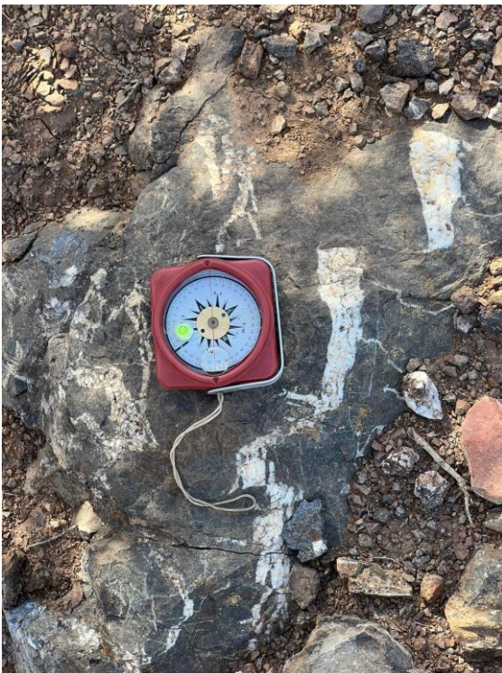
Figure 4 – Outcropping oxidised stibnite mineralisation
