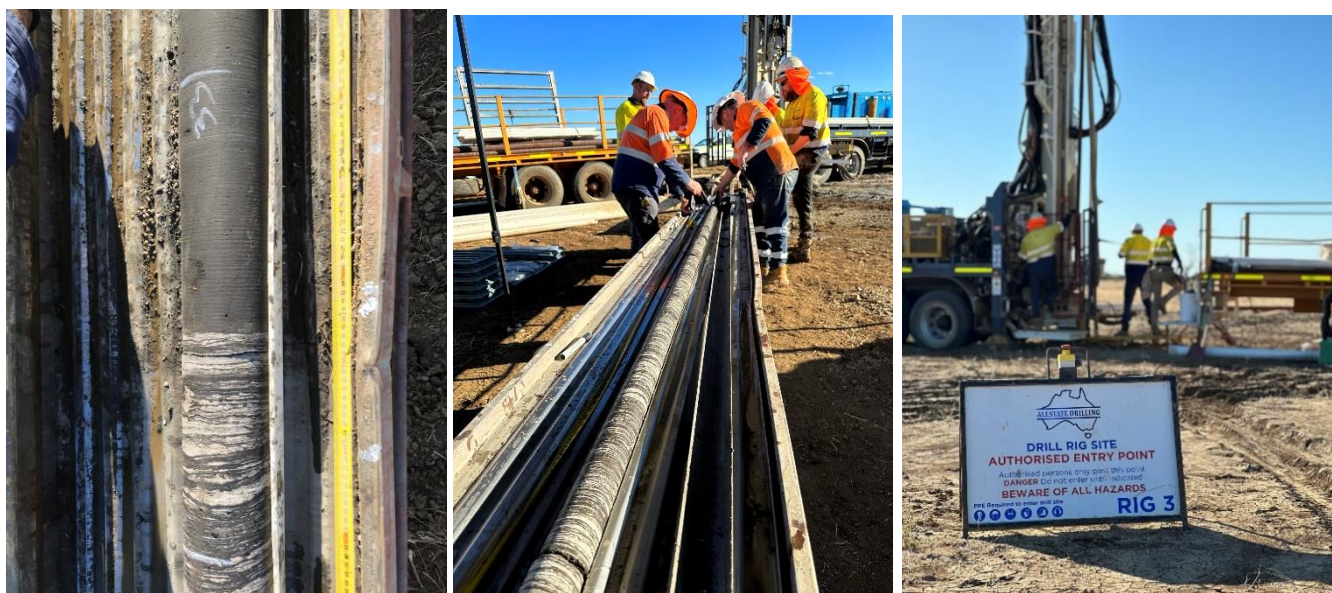
Images: Core sample showing transition point from coquina to oil shale stratigraphic units, core recovery, All State Crew.
