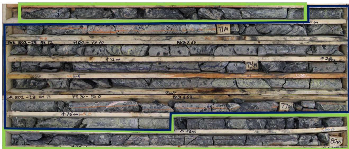
Figure 6: Faulted interval in drillhole GKI-002 characterised by successive moderately to strongly chloritized and argillised cataclastic fault cores (green box) separated by a damage zone (blue box) displaying anastomosing protocataclastic fabric and fractures.
