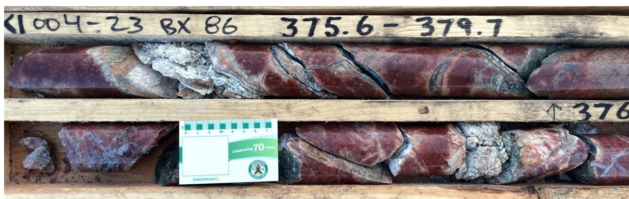
Figure 4: Close-up of strongly fractured hematized interval intersected in drillhole GKI-004. Deformation is characterized by an extensive network of microfractures, open fractures, quartz veins, cohesive dark green cataclastic bands and incohesive centimetre scale breccias and gouges. A bleaching halo is commonly observed peripheral to the fractures and microfractures planes and gritty white fine grained clay matrix is noted in the incohesive breccia and gouges.
