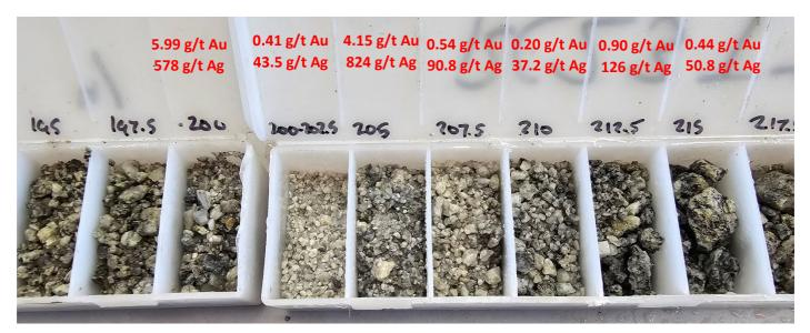
Figure 7: Mineralisation in RC23TT039 between 197.5ft – 215ft. Top contact defined by quartz-sulphide veining (25%) with lower veining levels and grey sulphide clays throughout remainder of interval.
