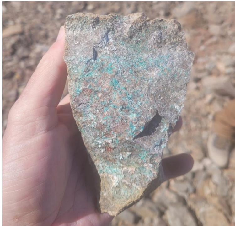
Figure 7: Copper oxide minerals in hand specimen from potassic altered porphyritic diorites at Ilo Este # containing approximately 1.5% to 2% copper oxide on the surface of the hand specimen. The presence of copper oxides in hand specimen indicates a mineral species only and should not be considered a substitute for analytical results. Visual estimates of mineral abundance should never be considered a proxy or substitute for laboratory analyses
