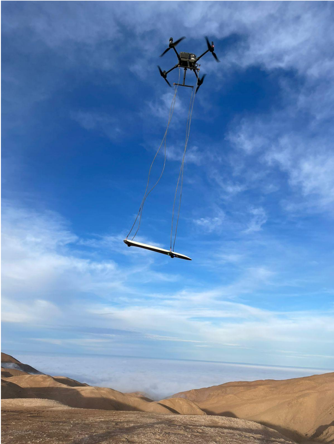
Figure 3: Drone magnetometry survey underway at Ilo Norte
