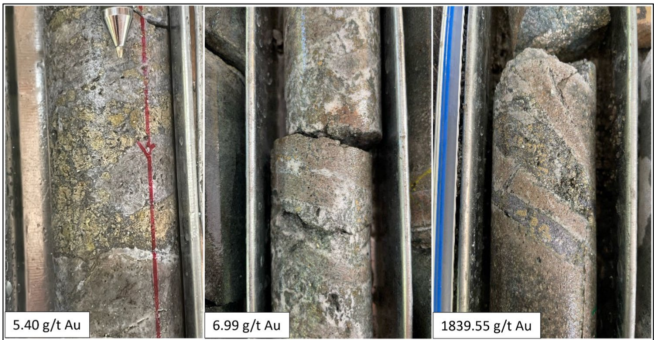
Figure 5. Example Mineralization from Zone 5 Grade Control Drilling. Left: URW3 lode. Monzonite hosted hydrothermal breccia with coarse grained sphalerite and pyrite (TGC-0056, 29.1 m). Center: Vuggy hydrothermal breccia with colloform silica, coarse grained sphalerite and pyrite, and strong potassic alteration halo (TGC-0067, 48.3 m). Right: Hydrothermal breccia with grey chalcedonic silica, coarse grained pyrite and sphalerite rimmed by fine grained sooty pyrite. Strong potassic alteration halo (TGC-0067, 49.0 m). Width of core is 4.76 cm in each photo.
