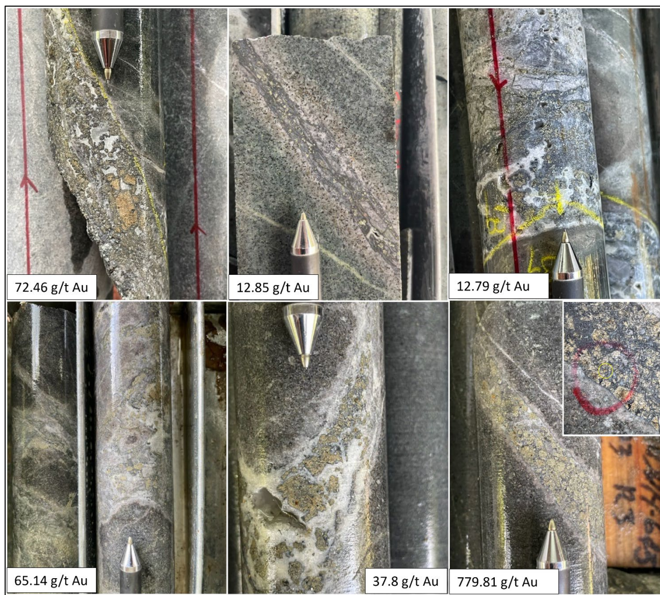
Figure 4. Example Mineralization from Zone 5 Infill Drilling. Top left: UR5 lode. Colloform quartz vein with abundant coarse grained honey sphalerite rimmed by fine-grained sooty pyrite (TUDDH-637, 162.0 m). Top center: UR2 lode. Narrow chalcedonic quartz vein with fine grained pyrite and sphalerite, weak potassic alteration halo (TUDDH-644, 220.3 m). Top right: Banded, vuggy and colloform chalcedonic quartz vein with coarse grained sphalerite and fine-grained pyrite and galena. Strong chocolate brown alteration halo (TUDDH-637, 220.3m). Bottom left: UR1/UR2 lodes. Wide variable white to grey silica vein with coarse grained sphalerite and pyrite (TUDDH-643, 243.9 m). Bottom center: UR1/UR2 lodes. Vuggy white silica vein with coarse grained sphalerite and pyrite (TUDDH-643, 247.6 m). Bottom right: UR1/UR2 lodes. Quartz-sphalerite-pyrite vein with abundant coarse-grained sphalerite and narrow potassic alteration halo. The inset image identifies a speck of visible gold within the yellow circle (TUDDH-643, 249.0 m). The examples of mineralization shown here are from the sample area reported in this release with full assay results included in the appendix. Pen used for scale.
