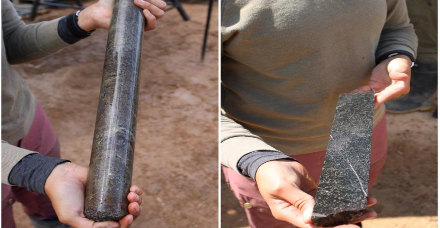
Figure 1: W56 prospect - (left) WL23-367 Massive Sulphides grading 1.35m @ 5.05% Ni from 227.2m and (right) net texture sulphides grading 4.4m @ 1.55% Ni from 247.1m.
