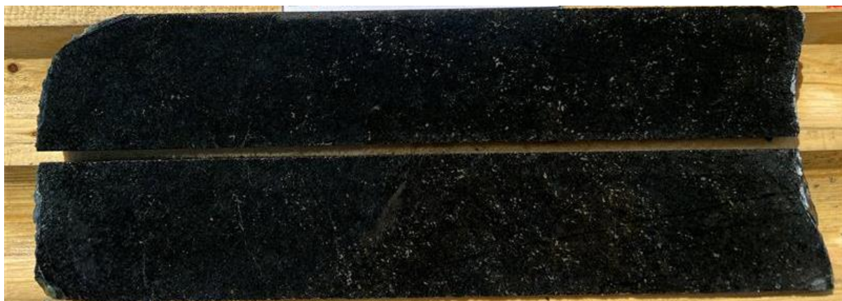
Figure 1: DDED23-131 interstitial to disseminated sulphide mineralisation at 270.2m
