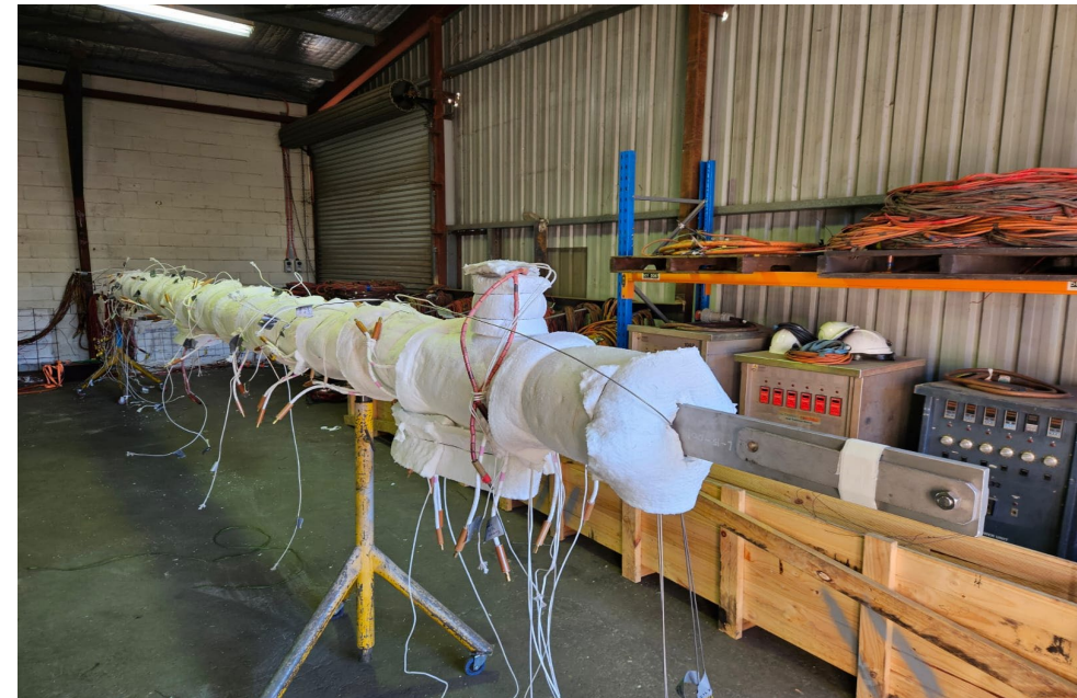
Heat exchanger successfully heat-treated prior to final assembly and delivery
