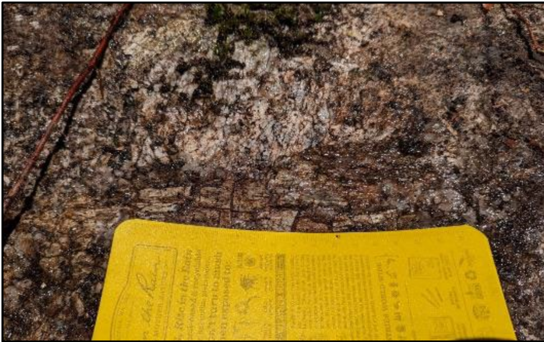
Figure 2 – Spodumene crystals in outcrop in the eastern section of Falcon Lake 1 (Table1; StationID: R23FL-PS06).
