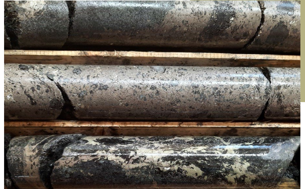
Discovery hole WAP22-003 interval comprises coarse grained pentlandite, chalcopyrite and pyrrhotite Source: Azmut Exploration
